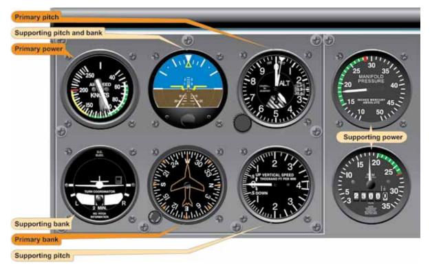
Figure 5-24. Straight-and-Level Flight (Reduced Airspeed Stabilized).
