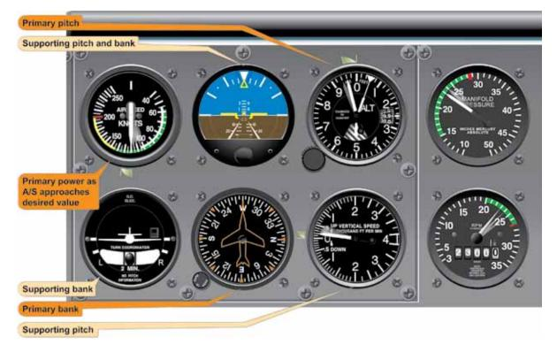
Figure 5-29. Level Off at Cruising Speed.
