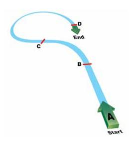
**Figure 5-43.** 80/260 Procedure Turn (Entire Pattern in Level Flight).
