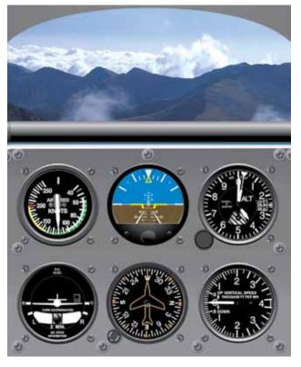
**Figure 5-3.** *Pitch Attitude and Airspeed in Level Flight, Normal Cruise Speed.*
