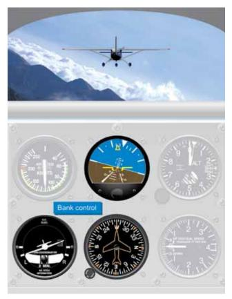
Figure 5-16. Instruments Used for Bank Control.
