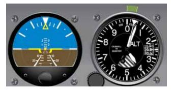
Figure 5-9. Altitude Error, Less Than 100 Feet.
