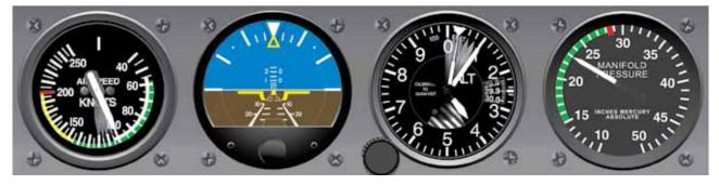
Figure 5-20. Airspeed Low and Altitude High—Lower Pitch.
