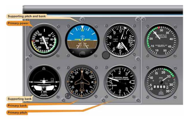
Figure 5-27. Stabilized Climb at Constant Rate.
