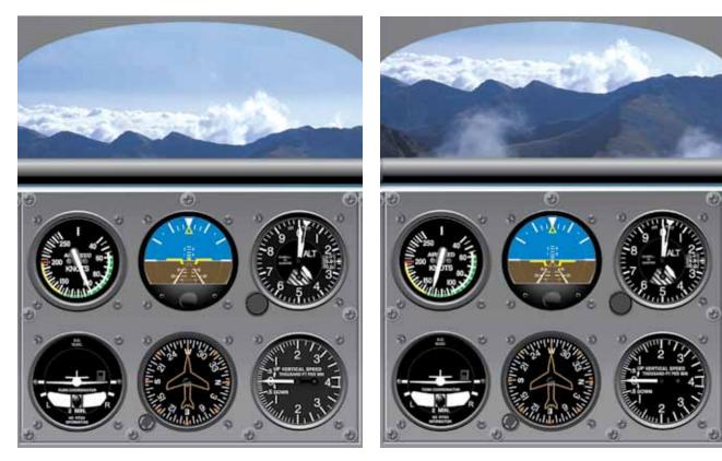
**Figure 5-1.** *Pitch Attitude and Airspeed in Level Flight, Slow Cruise Speed.*
