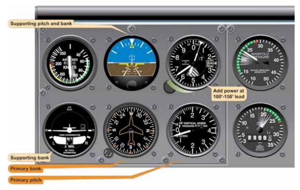
Figure 5-31. Level Off Airspeed Higher Than Descent Airspeed.
