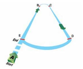
Figure 5-41. Racetrack Pattern (Entire Pattern in Level Flight).
