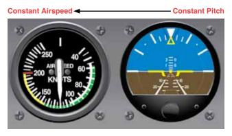
Figure 5-13. Constant Power Plus Constant Pitch Equals Constant Speed.
