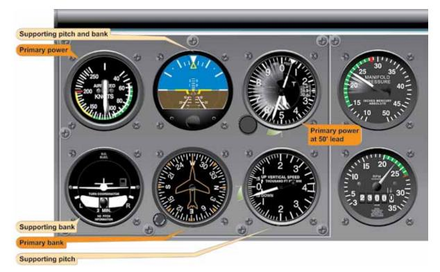
Figure 5-32. Level Off at Descent Airspeed.
