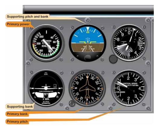
Figure 5-28. Airspeed Low and Vertical Speed High—Reduce Pitch.
