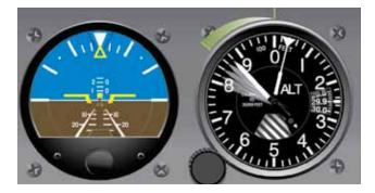
Figure 5-12. Pitch Correction, Greater Than 100 Feet—One Bar Correction Initially.
