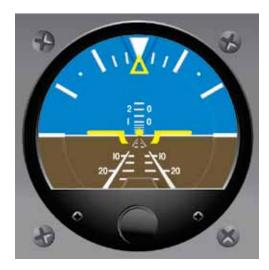
Figure 5-4. Pitch Correction for Level Flight, One-Half Bar Width.
