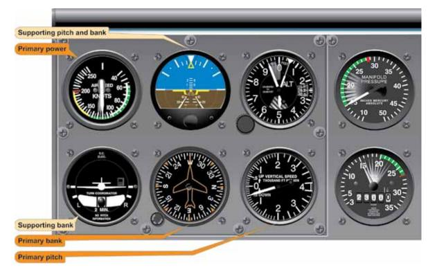
Figure 5-30. Constant Airspeed Descent, Airspeed High—Reduce Power.
