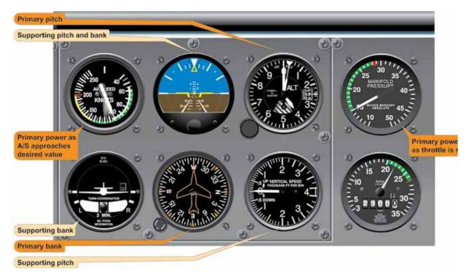
Figure 5-23. Straight-and-Level Flight (Airspeed Decreasing).
