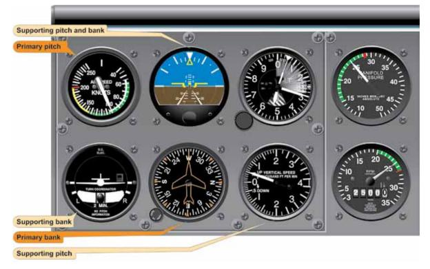
Figure 5-26. Stabilized Climb at Constant Airspeed.
