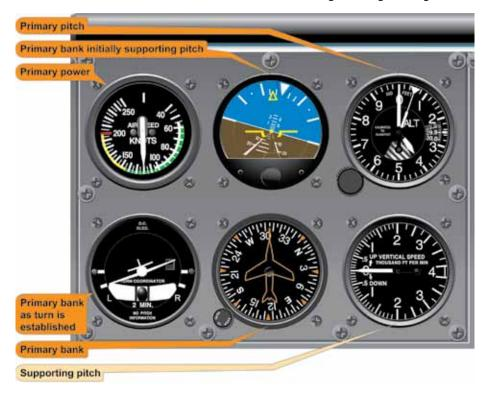
Figure 5-33. Standard Rate Turn, Constant Airspeed.
