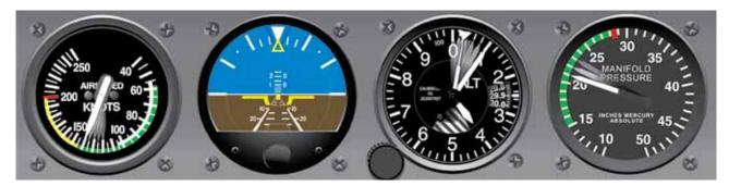
Figure 5-21. *Airspeed and Altitude High—Lower Pitch and Reduce Power.*
