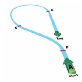
**Figure 5-42.** *Standard Procedure Turn (Entire Pattern in Level Flight).*
