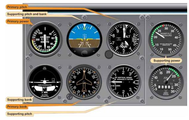
Figure 5-22. Straight-and-Level Flight (Normal Cruising Speed).
